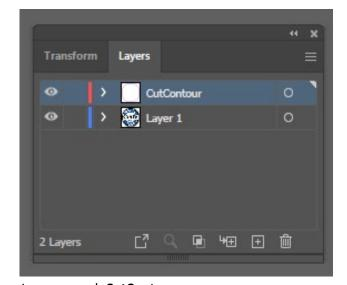
Layer named: **CutContour CutContour** layer must be the top layer.
