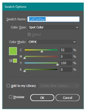
Custom Swatch named: **CutContour**The **CutContour** swatch can be any color, but it MUST be of a Spot Color type.
